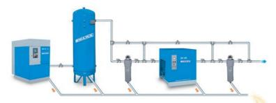
As an example, if a compression system with a refrigerant dryer with a capacity of 20 m³/min, 10 bar were to operate at 60% full load, two shifts a day, for 220 days/year, at a room temperature of 25 °C and 70% relative humidity, its condensate production would be about 39,000 litres/year.
